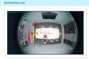
2) Ensure the detection target can pass through the detection line completely. It's recommended that draw the detection line perpendicular to the In/Out direction, and make the line on the center of detection area without other objects around.
