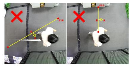
3) A redundant identification area needed to be left on both sides of the detection line for the target. This is to ensure that the sensor has stable recognition and tracking of this target before it passes the detection line, which will make the detection and count more accurate.
