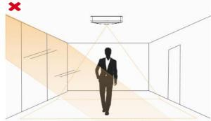
• Make sure there are no moving objects interfering in the counting area. For example, do not install the sensor too close to a door.
