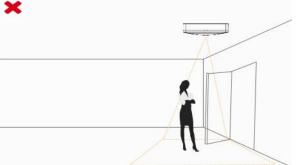
• Avoid installing the sensor near a mirror or avoid drawing the line to the mirror.
